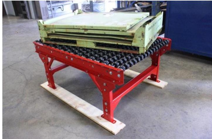
The product selected was a 32" Max Performance roller with the Rotacaster R2-0484-99 wheel on 2" centers. Rollers were installed on 3" centers.
